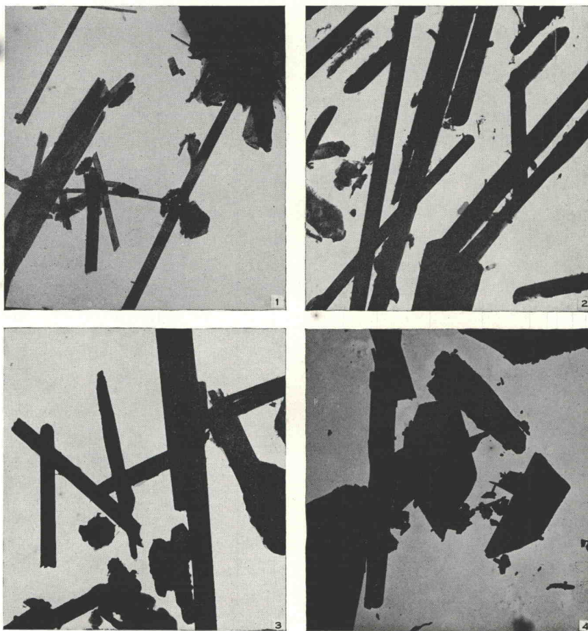
Electronmicrographs ( \times 10,000 ) of graphitic chalcogenides : 1, \text{ZrS}_3 ; 2, \text{ZrSe}_3 ; 3, \text{ZrSe}_2 ; 4, \text{ZrTe}_3 .
